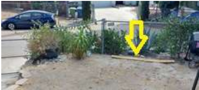
Path of plastic pipe. Depth about 3 ½’.
